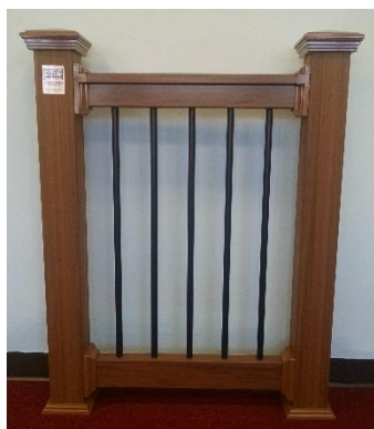
Woodgrain PVC T-Rail and 2" x 3.5" Woodgrain Bottom Rail with ¾" Round Black Aluminum Balusters
